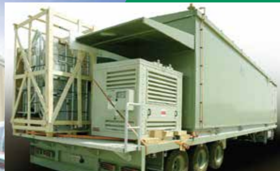
Mobile switch gear container on a trailer
