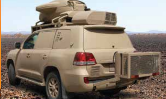
VSAT Communication Station on a Land Cruiser
