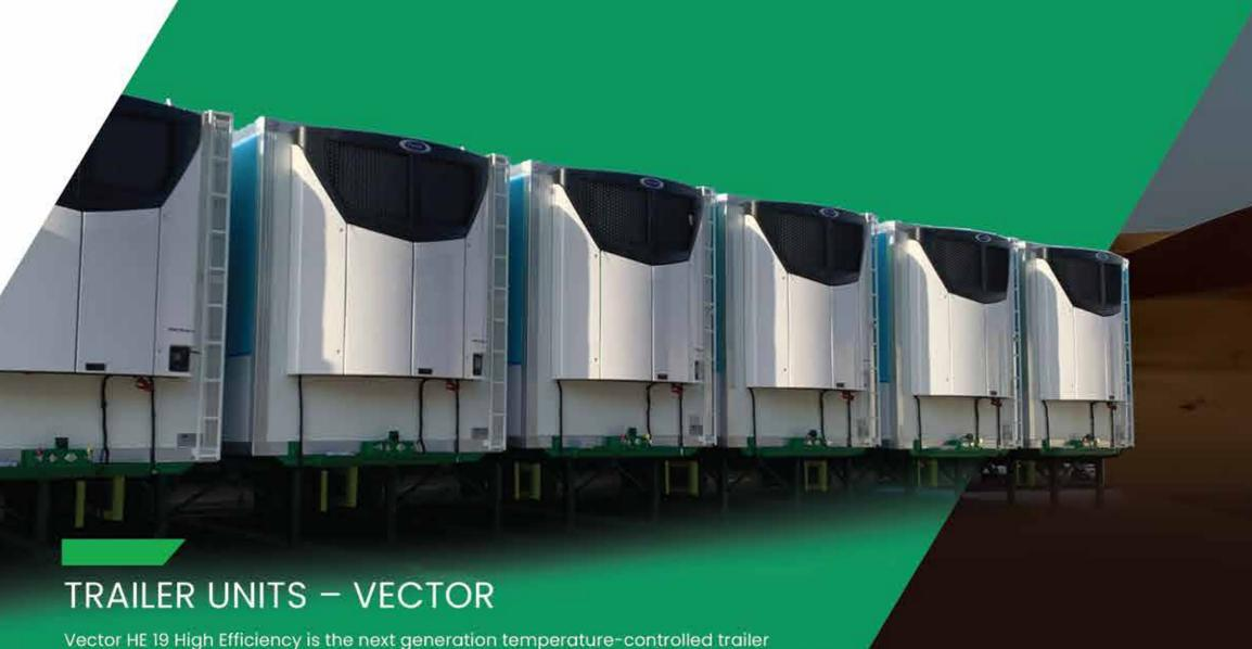
Vector HE 19 High Efficiency is the next generation temperature-controlled trailer system. The unit combines experienced technology, like the all-electric architecture of the E-Drive, with new additions designed to significantly improve performance and efficiency. Operators will benefit from improved fuel consumption by up to 30 per cent, reduced unit weight by 10 per cent and a noise emission lowered by 3dB(A).
