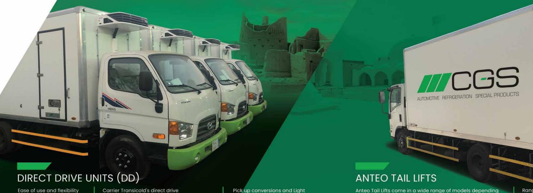
Carrier Transicold's direct drive refrigeration units are specifically designed for the transportation of fresh or frozen goods in small-to-medium sized delivery vehicles.
